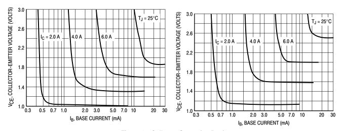
Figure 10. Collector Saturation Region
