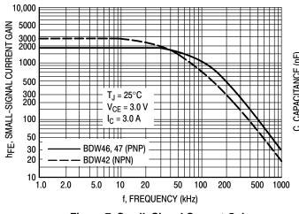
Figure 7. Small-Signal Current Gain
