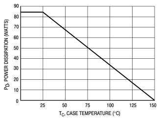
Figure 1. Power Temperature Derating Curve
