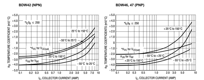
Figure 12. Temperature Coefficients
