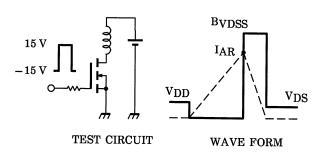
$$\begin{aligned} &R_G = 25~\Omega \\ &V_{DD} = 90~V,~L = 25.5~mH \end{aligned} \qquad E_{AS} = \frac{1}{2} \cdot L \cdot I^2 \cdot \left(\frac{BV_{DSS}}{BV_{DSS} - V_{DD}}\right) \end{aligned}$$
