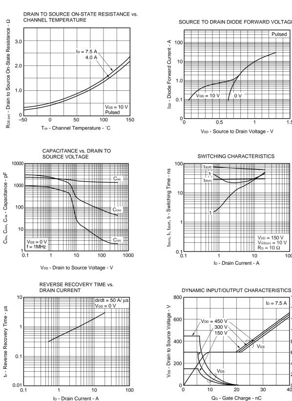
SOURCE TO DRAIN DIODE FORWARD VOLTAGE
